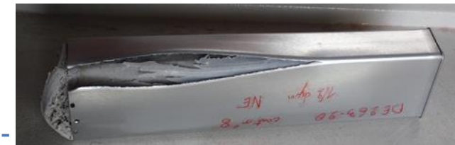
MTV ageing hardened tests without seal
