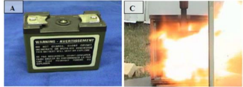
Lithium-thionyl chloride battery – penetration by a nail – explosion 5 min after the fire started
